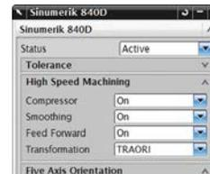
*A special menu in NX CAM enables you to select key functions on the Sinumerik controller.*
