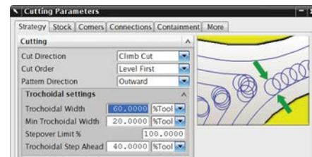
*The trochoidal cutting pattern in NX automatically prevents you from exceeding permissible cutting conditions based on user-specified criteria.*
