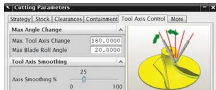
*Tool axis parameters* enable you to create optimized 5-axis tool path.
